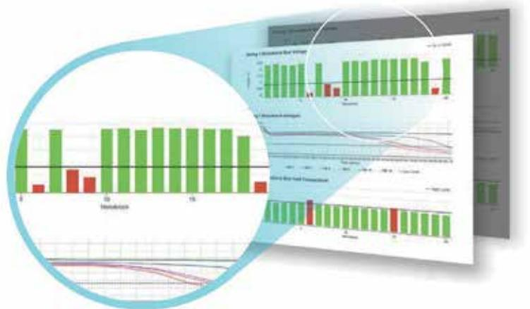
All discharges are reported, issues recorded and recommended maintenance actions are listed. Between reports the PowerShield battery monitoring system will continue to notify you directly of any alarms where immediate onsite action is needed.
