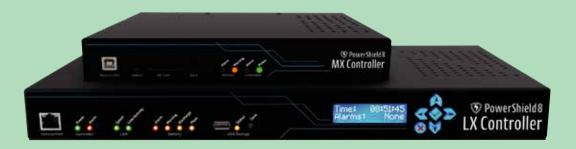
Controllers are smart devices that collect, analyse and store the battery measurements retrieved from the Lithium BMS. Continuous, fast data sampling in all string states (charge, discharge and idle) allows the Controller to initiate event logging and provide real-time battery visibility and status.
